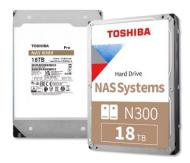
The 18TB N300 is a 9-disk helium-sealed conventional magnetic recording (CMR) drive that leverages Toshiba's new innovative Flux Control Microwave-Assisted Magnetic Recording (FC-MAMR™) technology. FC-MAMR™ advances CMR capacity to 18TB and delivers increased density per platter over previous designs. This is the 3rd generation to use Toshiba's pioneering 9-disk helium-sealed mechanical design.
